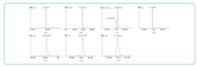
Fig. 2 Mass spectra of CH<sub>4</sub>, H<sub>2</sub>O, N<sub>2</sub>, CO, O<sub>2</sub>, Ar, Kr, Xe (enlarged near peak regions)
