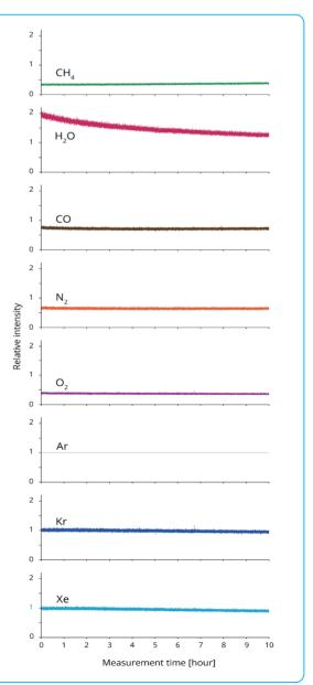
Fig. 3 Mass chromatogram of CH<sub>4</sub>, H<sub>2</sub>O, N<sub>2</sub>, CO, O<sub>2</sub>, Ar, Kr, Xe
