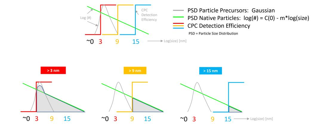
Size selective condensation growth down to 3 nm enables both Particle Precursor and Native Particle distributions to be measured.
